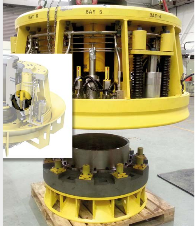
MAGNUMS allow for emergency quick disconnection of the pipelines from the oil rigs
